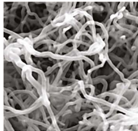
FIGURE 1.1.2 These carbon nanotubes have different properties from other materials made from carbon such as charcoal, graphite and diamond.
