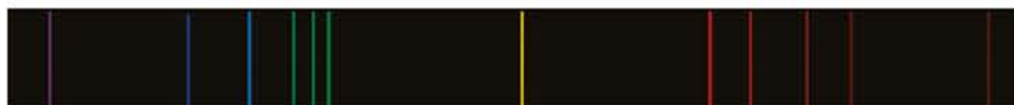
FIGURE 1.5.3 The emission spectrum of helium is made up of lines ranging from violet to red in colour.
