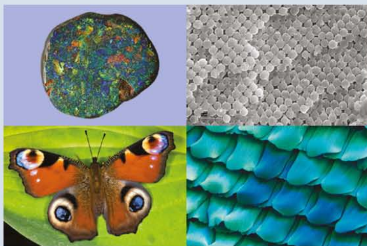
FIGURE 1.1.3 (Top) An opal is made of tiny spherical nanoparticles of silica. (Bottom) The colour of a butterfly's wing is due to nanostructures in the wing.
